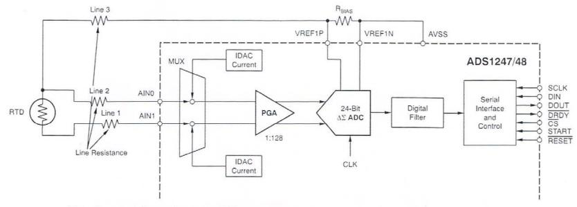
Note: R<sub>BIAS</sub> should be as close to the ADC as possible.
