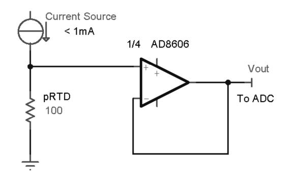
Read AN 687 for more details (e.g. current excitation circuit): http://ww1.microchip.com/downloads/en/AppNotes/00687c.pdf http://www.control.com/thread/1236021381 on 3-wire RTD
