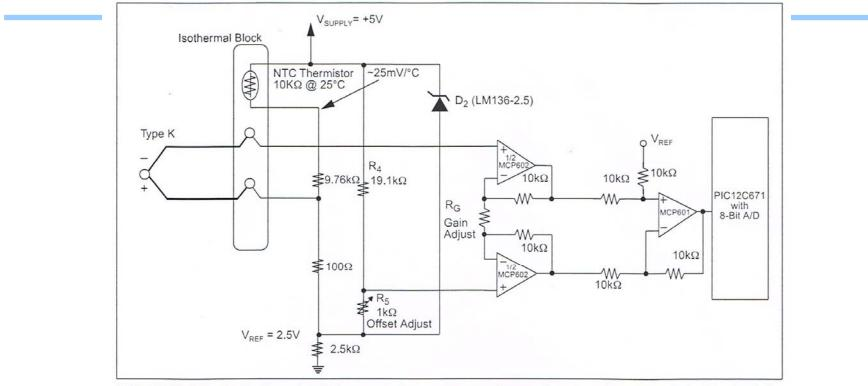
FIGURE 15: This circuit will provide 8-bit accurate temperature sensing results using a thermocouple. In this circuit, the A/D Converter is included in the PIC12C671 microcontroller.
