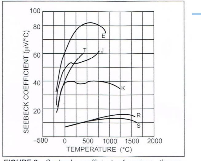
FIGURE 2: Seebeck coefficient of various thermocouples versus temperature
